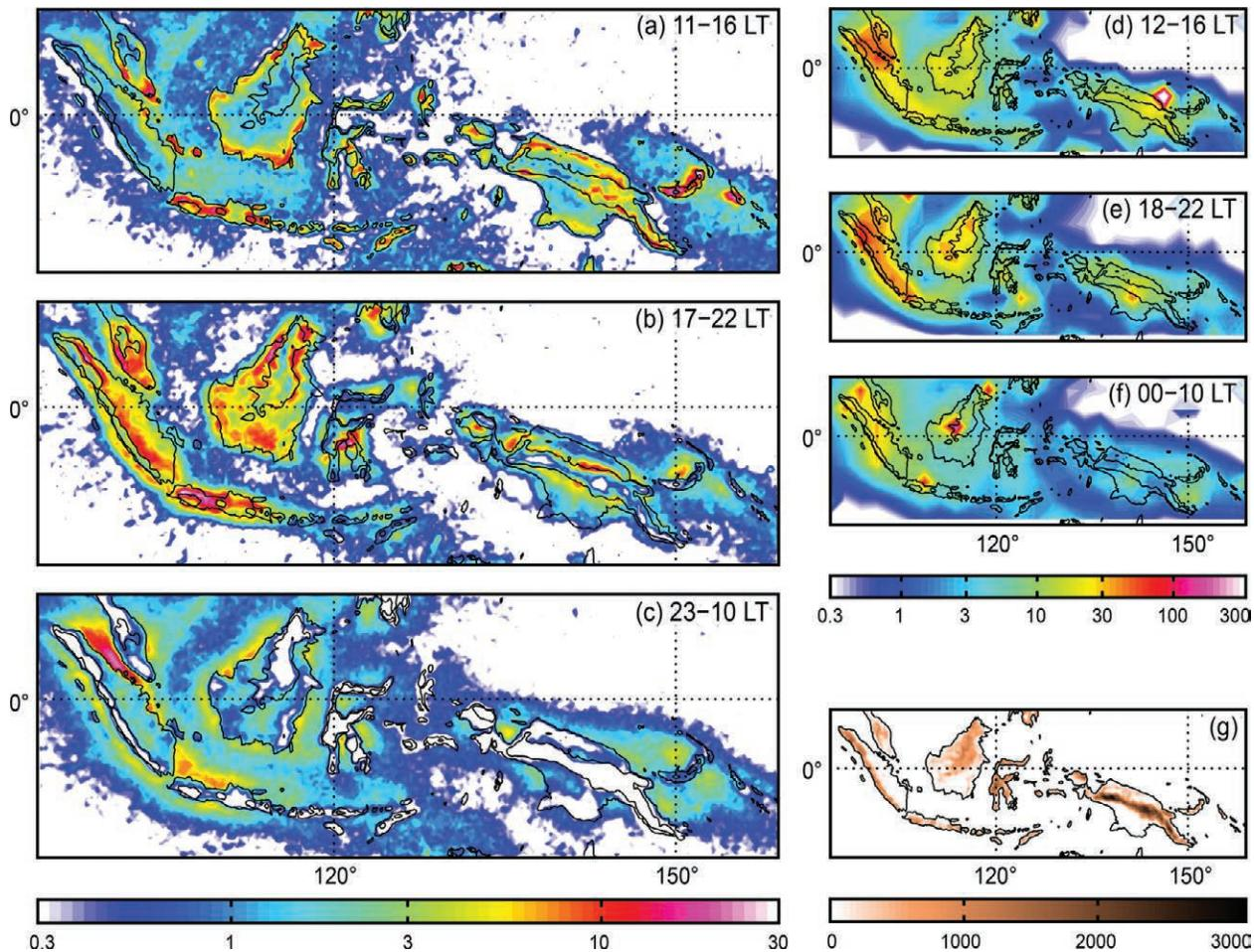
FIG. 6. (a)–(c) WWLLN lightning stroke frequency ( $\text{km}^{-2} \text{yr}^{-1}$ ; hourly,  $0.25^\circ \times 0.25^\circ$  resolution) and (d)–(f) LIS/OTD lightning flash frequency ( $\text{km}^{-2} \text{yr}^{-1}$ ; two hourly,  $2.5^\circ \times 2.5^\circ$  resolution) for indicated time intervals during all months. Local time given for Singapore. Black contours indicate the 500-m elevation. (g) Elevation (m).
