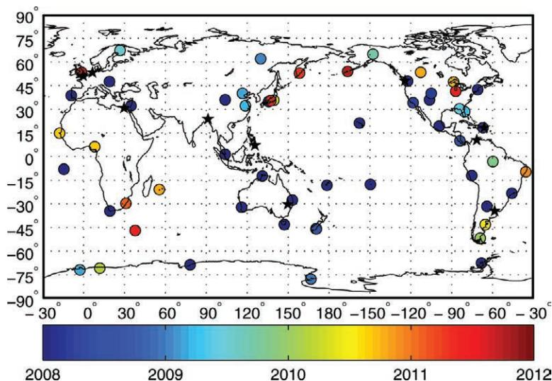
**FIG. 1.** Location of WWLLN sensors, color coded according to the date each was established. Stations established prior to 2008 are shown in dark blue; black stars indicate stations established 2012–present.
