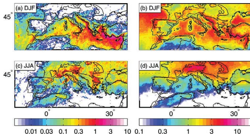
**FIG. 5.** (a),(c) WWLLN lightning stroke frequency ( $\text{km}^{-2} \text{yr}^{-1}$ ) and (b),(d) TRMM 3B42 precipitation ( $\text{mm day}^{-1}$ ; both at  $0.25^\circ \times 0.25^\circ$  resolution) during (a),(b) DJF and (c),(d) JJA. Black contours indicate the 500-m elevation.
