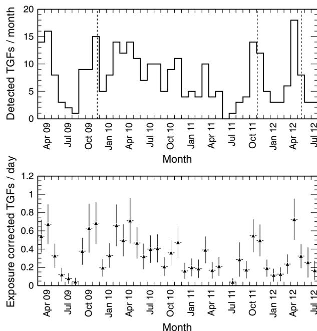
**Figure 1.** (top) AGILE TGF monthly detection rate. Dashed vertical lines, from left to right, mark AGILE entering spinning mode, and two successive MCAL energy threshold adjustments. (bottom) Daily TGF detection rate corrected for AGILE MCAL exposure.
