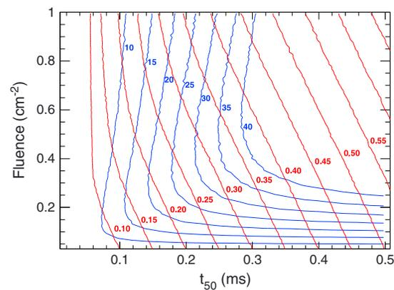
**Figure 6.** Contour plots of the number of detected counts  $N^{\text{obs}}$  (blue curves) and measured duration  $t_{50}^{\text{obs}}$  (red curves) in the true (duration, fluence) parameter space, assuming the dead time model discussed in the text.
