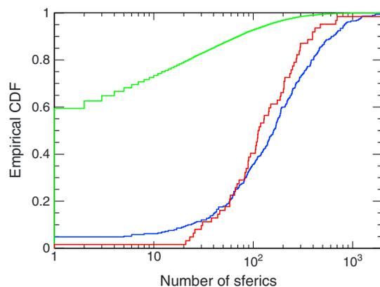
**Figure 11.** Empirical cumulative distribution functions (CDF) for the number of sferics detected within a radius of 600 km from the subsatellite point in a 20 min time interval centered at the TGF time ( $N_{600}$ ) for AGILE TGFs (blue curve), a sample of the new RHESSI TGFs with latitude lower than  $10^\circ$  in absolute value (red curve), and a sample of AGILE positions extracted at random times (green curve).
