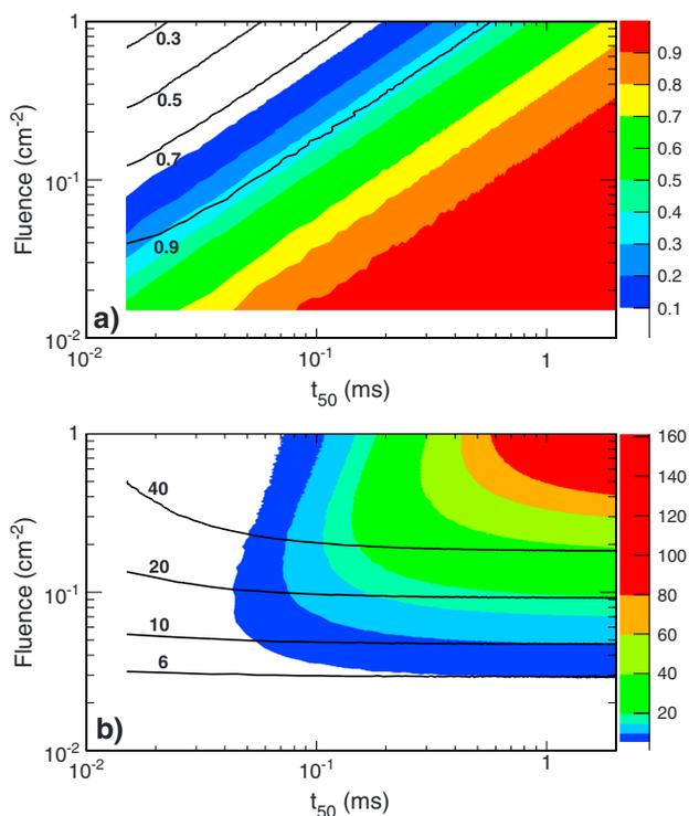
**Figure 2.** (a) Efficiency  $\epsilon$ , i.e., the fraction of detected counts; (b) number of counts detected  $N^{\text{obs}}$  after dead time is taken into account, as a function of the true TGF duration and fluence, for TGFs detected  $60^\circ$  off-axis angle. Color scale: AC-induced dead time only. Black line contour: MCAL-induced dead time only.
